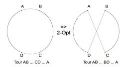
Figure 3.1: Exchange step of 2-opt algorithm
