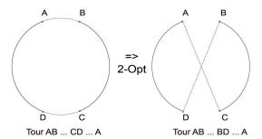
Figure 2.1: Edge removal and reconnection of 2-opt algorithm
